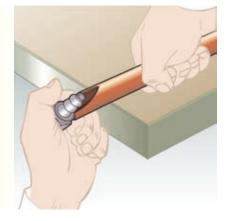
2. Grip hose and give a sharp down-ward tug to disengage from fitting.
