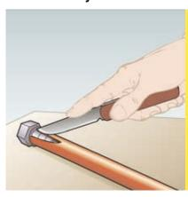
1. Cut lengthwise along a line at approximately a 20 angle from centre line of hose. The cut should be approximately 1" long. Be careful not to nick barbs when cutting the hose.
