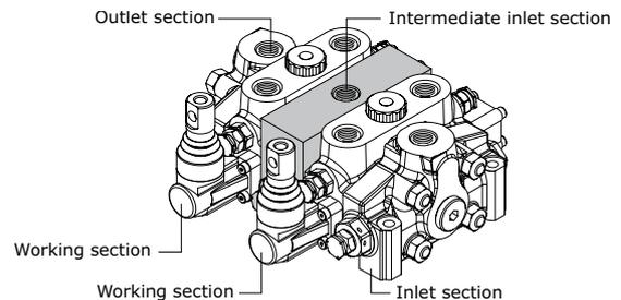
**Complete configuration samples for HC-D4/2 with intermediate inlet section (BV)**
