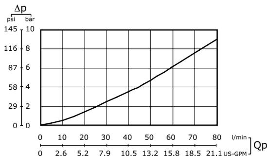
**Anticavitation check valve curve**
