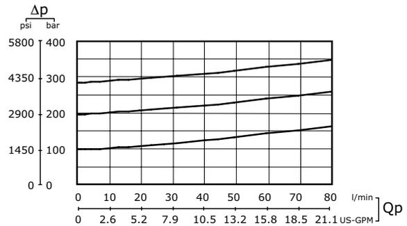
**Main anticavitation check valve curve**
