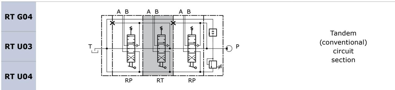
When the spool is operated it intercepts the switch gallery by diverting the flow of oil to service port A or B. The Tandem circuit is powered by the switch gallery thus permitting the use of just one work section at a time. The section downstream from the tandem section that has been actuated does not operate, the upstream section has priority.
