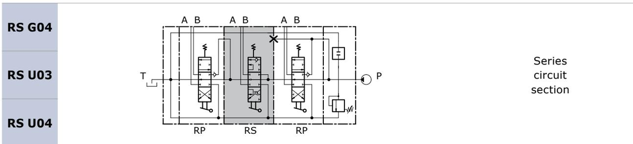
When the spool is operated it intercepts the switch gallery by diverting the flow of oil to service port A or B. The oil that flows back from the actuator is carried to the switch gallery thus making it available to the service ports downstream from the series section. The pressure drop downstream is added to the pressure drop of the section itself.
