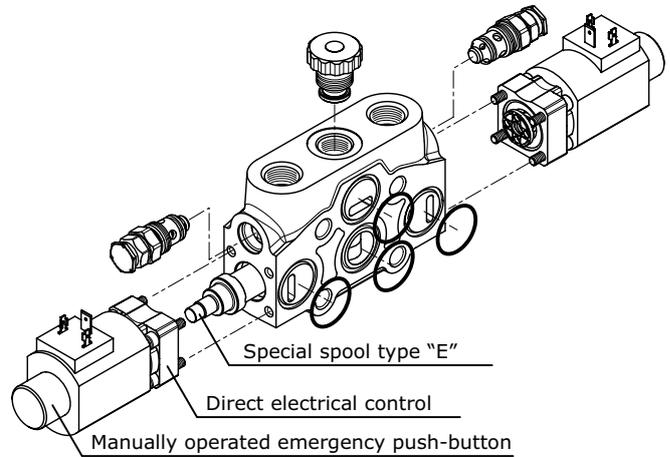
The H036 and H037 direct electric controls come as two kits each including a: coil, spring, solenoid and adapter. **The direct electric controls use a type E special spool.** The D4 control valve body is the standard type normally used for manual controls. The ON-OFF Electric Control kit includes a manually operated emergency push-button.
